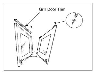
3. Hold the door glass securely with one hand, before removing the screws completely with the other hand.
